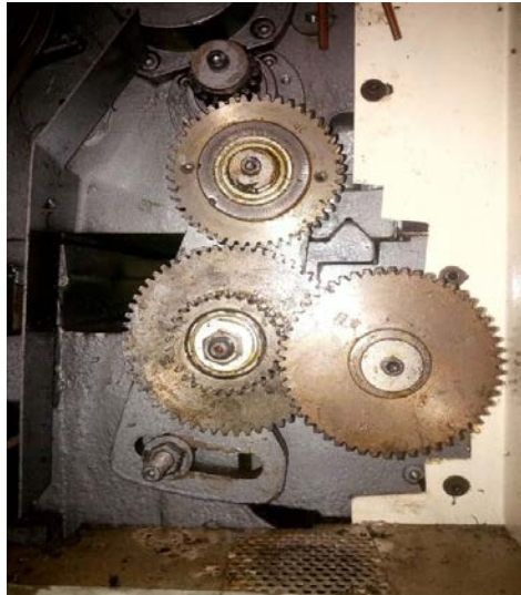
Figure 3.1- Lathe Machine Gear Mechanism
